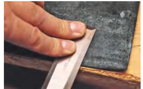
▲ It does work well enough but the leather is best bonded to a board
